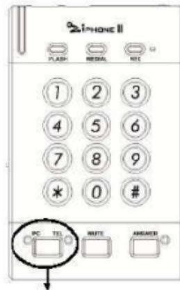
PC/Tel switch between PC (green LED) and TEL (red LED) mode
